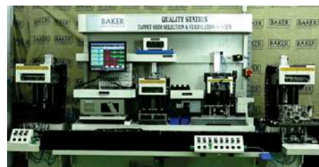
Shim & Spacer Cylinder Head Tappet Shim Selection
